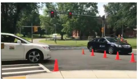
A Tampa vehicle (white) receives an IMA alert while trying to enter an intersection when a New York City vehicle (black) with the right-of-way passes through.
