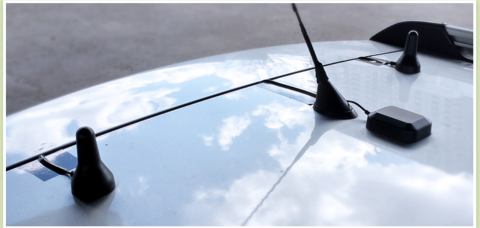
Three antennas on the roof of an SUV (near existing radio antenna)
