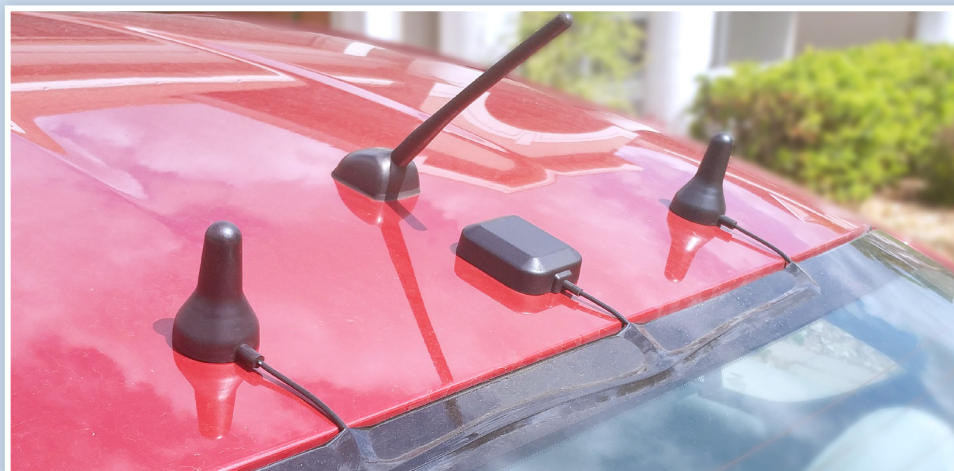
Three antennas on the roof of a sedan (near existing radio antenna)
